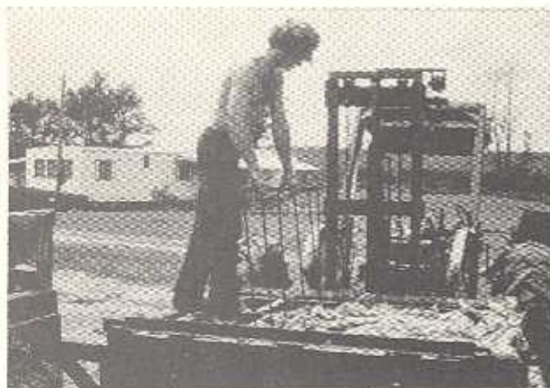
Figure 6. Tine bars being placed in loaded container.
