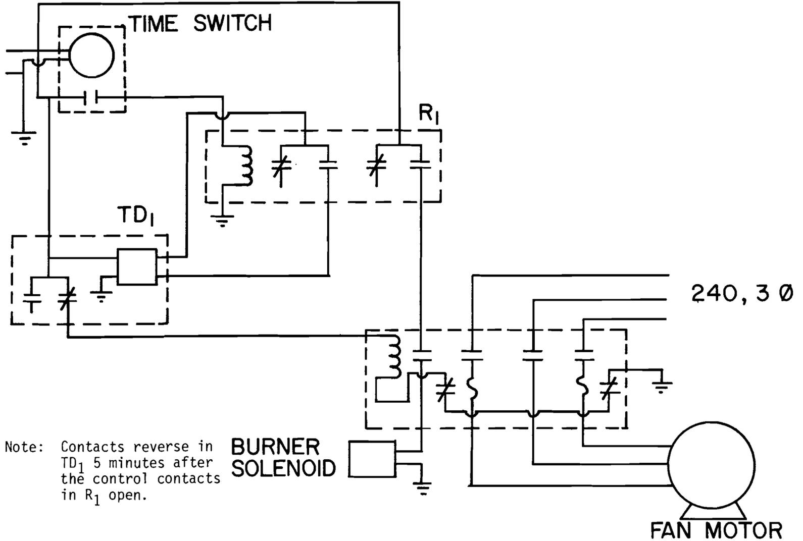
Note: Contacts reverse in TD<sub>1</sub> 5 minutes after the control contacts in R<sub>1</sub> open.
