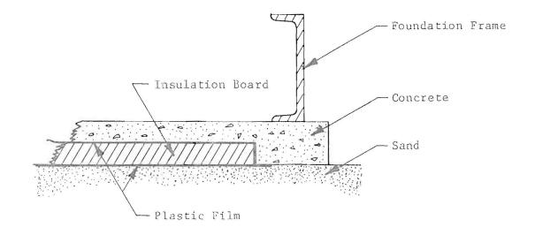
Figure 2. Insulation of foundation slab from the ground. (All dimensions in inches.)
